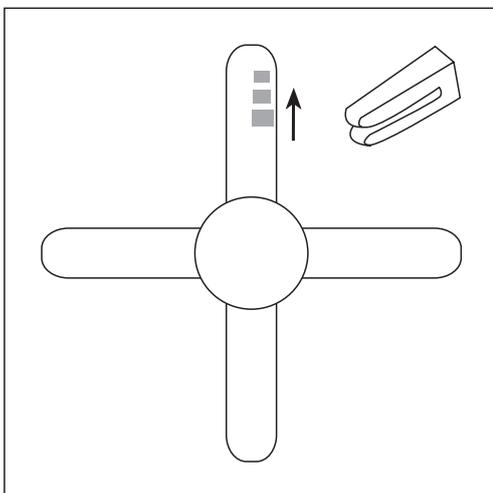
Place the clip on the blade that needs the counterweight and try the best place to place it, from the center to the tip of the blade, until the wobble disappears.
