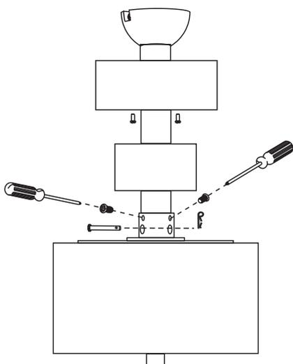
1. Thread the suspender through the suspended clock and coupling cover .
